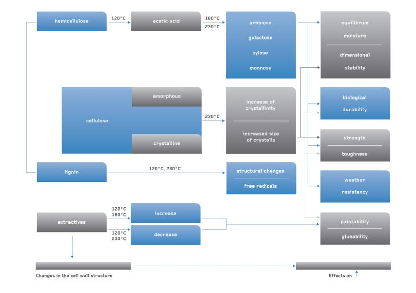
Reaction mechanism of thermally modified wood (source: VTT).
